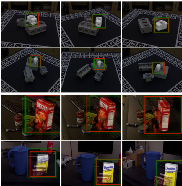
Fig. 7. Visualization of estimated poses on the T-LESS dataset (first two rows) and the YCB Video dataset (last two rows). Ground truth bounding boxes are red, green bounding boxes are particle RoIs, and the object models are superimposed on the images at the pose estimated by PoseRBPF.
